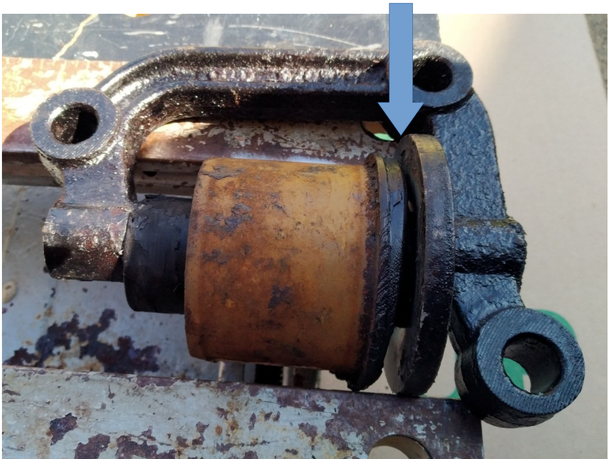
Old bush in place after old paint removed from shim. Note: some distortion on bush due to heating to remove
