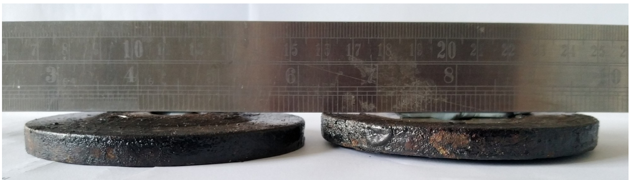
Shims to be shot blasted and painted
