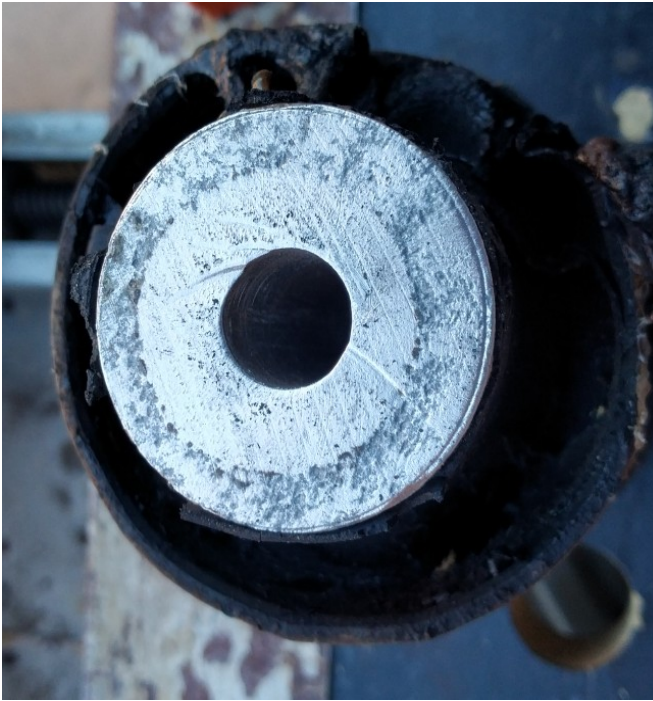
Old bush after cleaning – end against outer side bracket
