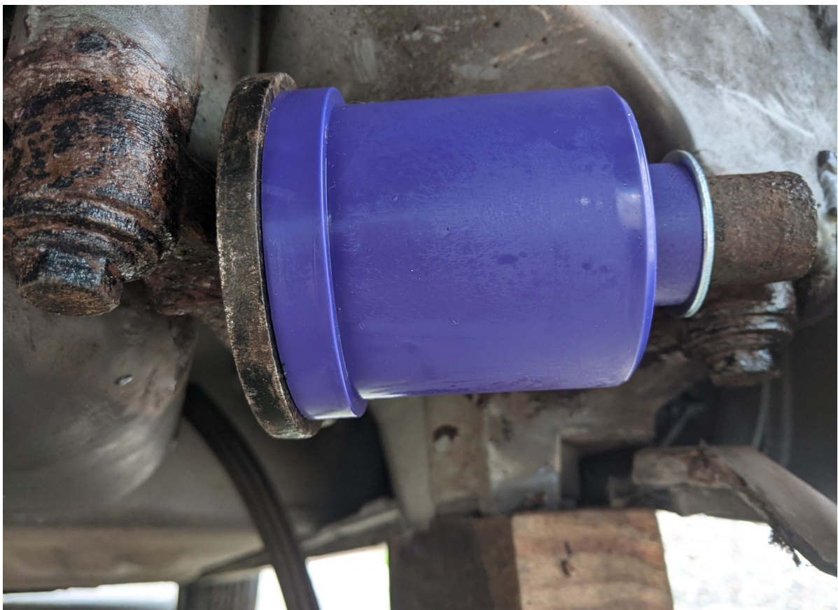
Stan's Powerflex bushes trial fit. Note left hand side is flush against the shim.
