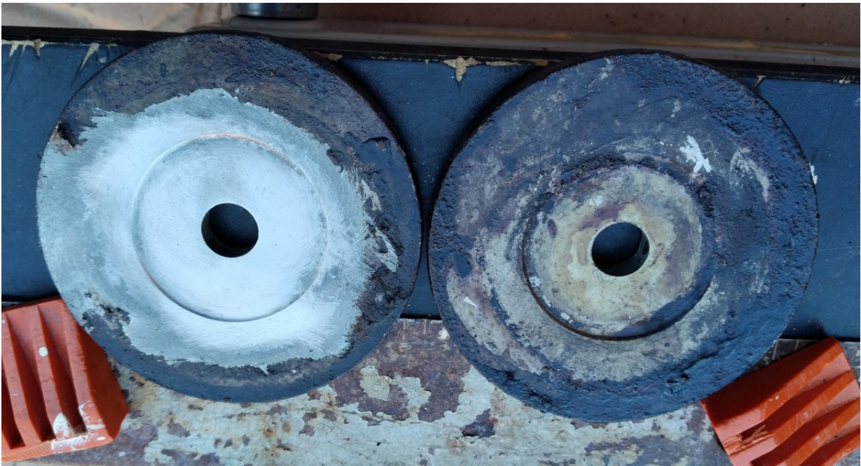
Paint removed from 1 shim - inner side against bush
