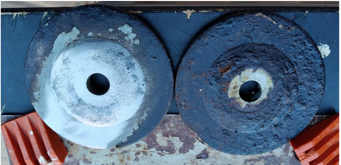
Paint removed from 1 shim - outer side against bracket
