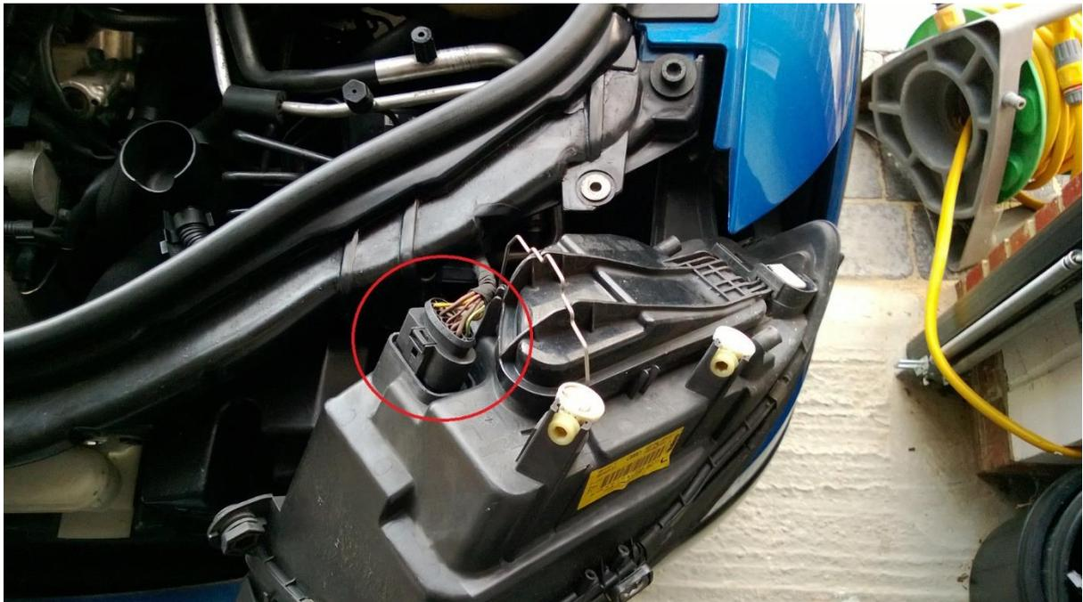
Having removed the light completely you should be able to see into the engine bay. Located at the back is a nice silver strip, this seems to me to be the best place to secure the ballast unit to.
