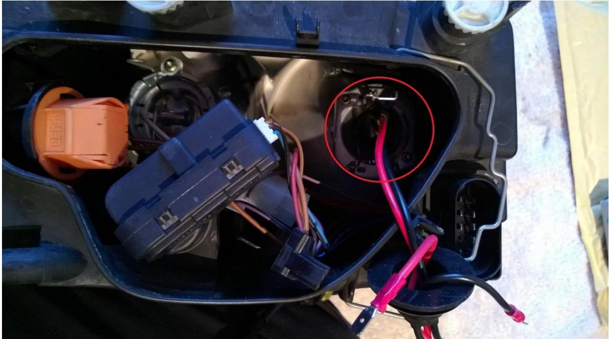
From the new HID bulb should be two wires, each with a spade connector on the end, they should be black and red. Find these and insert the two spade connectors into the existing light connector, they should fit in without much pressure. Ensure they are not touching each other or the unit will short circuit.
