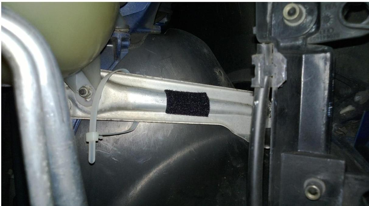
Once happy with the location, I stuck the ballast unit to the Velcro to test the location and length of wires was sufficient so it would reach the back of the head light.
