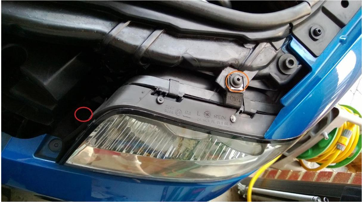
Now disconnect the wiring to the head light via the plug on the back, be careful not to damage the plug or socket.
