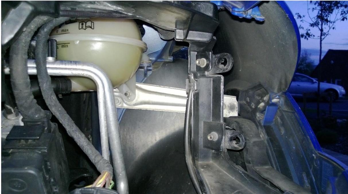
Rather than drill a hole and secure the ballast via a nut and bolt, I figured they might need to be removable so decided to secure mine with Velcro and cable ties. The Velcro to ensure the ballast didn't jump about and the cable ties to secure it to the Velcro.
