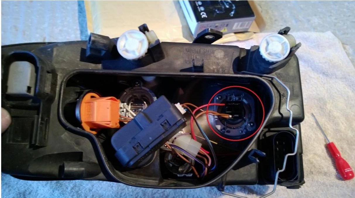
To do this, move the spring clip holding the bulb in place to one side and lift the bulb out, there should be little resistance on the spring clip and no resistance on the bulb.
