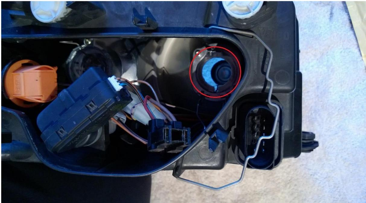
With the bulb removed, its time to place the new HID bulb in the hole, make sure you don't touch the side of the bulb or the glass, only hold it by the base. Once seated, secure the bulb in place with the spring clip, ensuring its locked down correctly.
