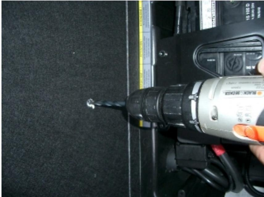
8) Because of the shape of the bracket you also need to hollow out an area around the small hole for this to fit with a carpet knife or similar.
