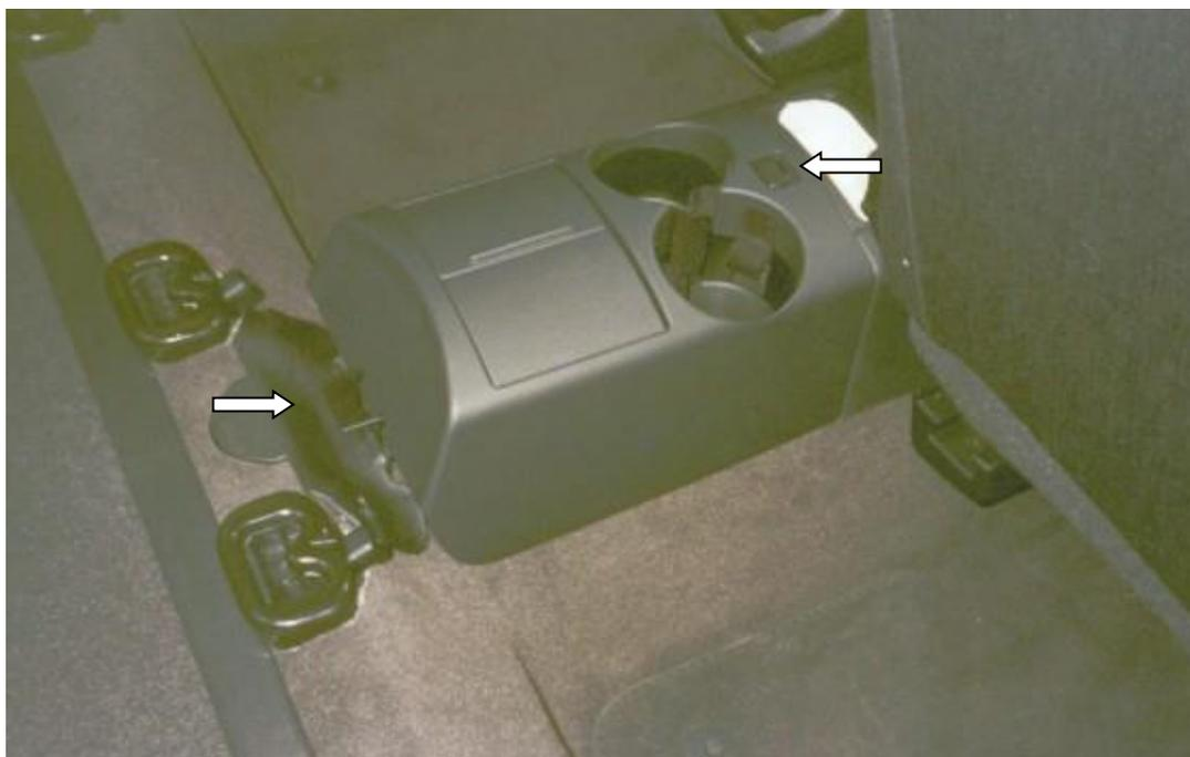
11. Remove drinks holder by pressing the button and then lifting the front end (Photo above).
