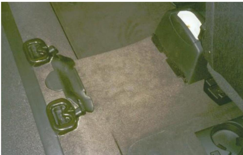
9. Push the front bracket under the rear of the centre console again must click (I had 2 supplied only one would fit the drinks holder the one without the 2 prongs) (photo below).
