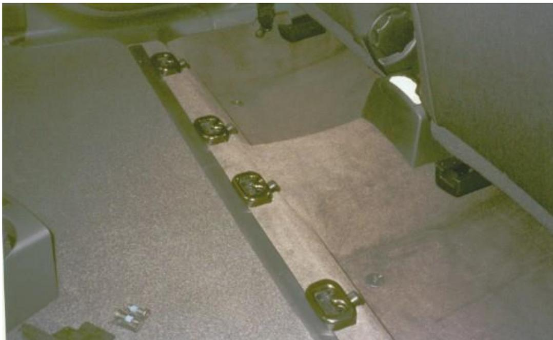
3. Remove plastic trim (push fit) with flat screwdriver (secured in 4 locations) (Photo below).
