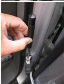
Use a punch and a hammer totap the the door pin downwards
