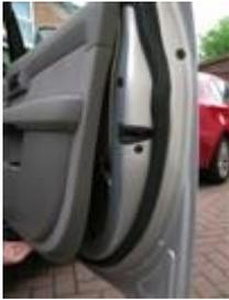
Pull the bottom of the door card away like this...You then bring the door card up -it hooks just below where the window scraper seal is
