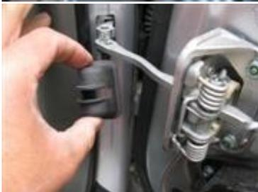
As all good manuals say, reassembly is the reverse of the disassembly - Don't forget the rubber cover before tapping the door pin back in
