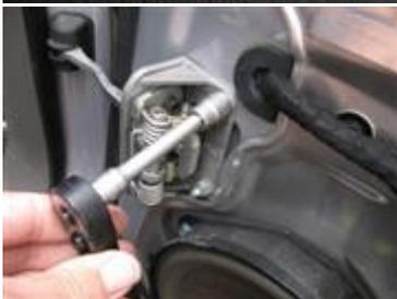
remove both 10mm nuts on the door strap assembly
