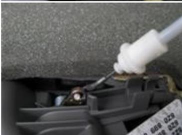
.....by simply pulling the white plastic holder and unhooking the cable end
