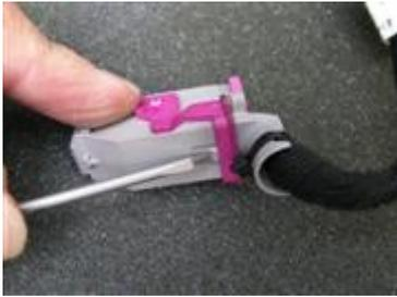
You can see here the tab you'll need to press with a small bladed screwdriver to release the pink tab.
